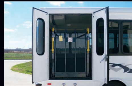
Optional double wheelchair door with top mounted gas shocks to hold door open in windy conditions
